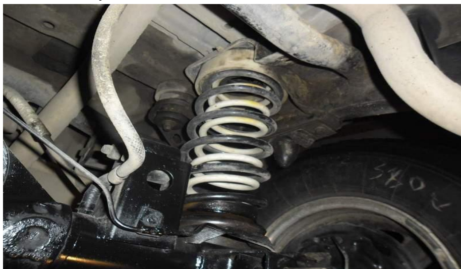
2-rasm. Kichikroq purjinalarni o‘rnatish
