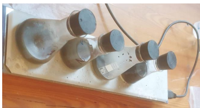
Figure 2.3- Hydrochloric acid leaching of MA copper slag with coal
