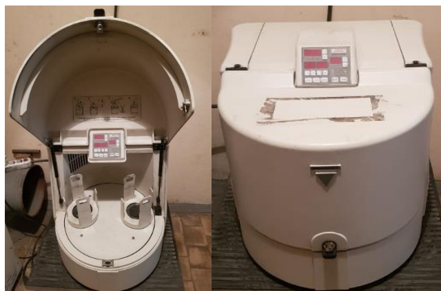
Figure 2.2- planetary ball mill used for mechanical activation of copper slag
