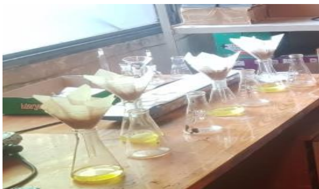
Figure 2.4- Filtration of solutions after hydrochloric acid leaching
