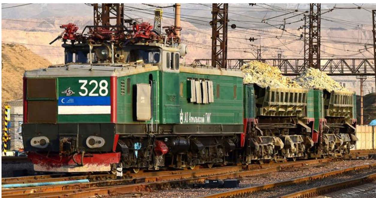
1 – rasm. “Olmaliq kon-metallurgiya kombinati” AJ ga qarashli PE2M-328 tortish agregati.
