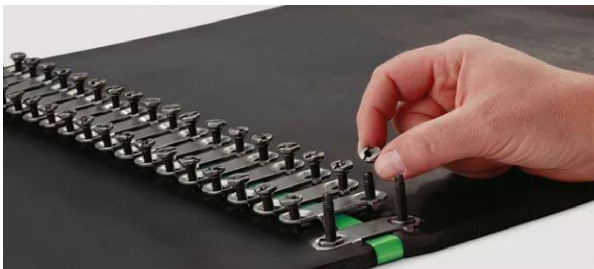
4-Rasm. Konveyer tasmasining mexanik ulash usuli
