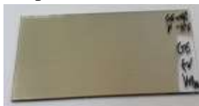
Figure 1-10. The fabricated sample coated on the glass with dual coatings Au-7nm / MgF 2 -135nm.
